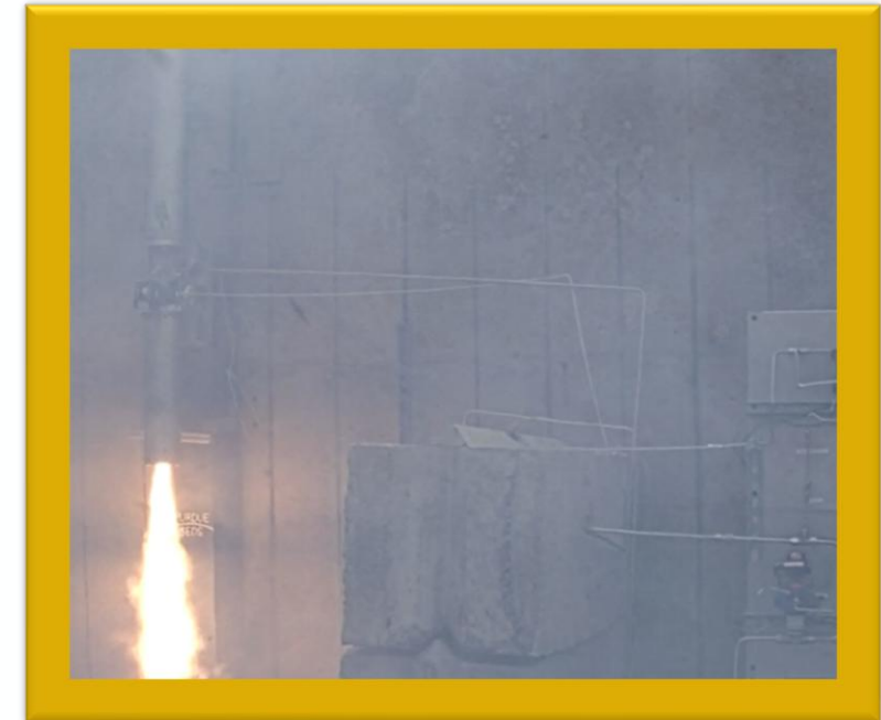
Hot firing our hybrid rocket engine at Zucrow Labs
